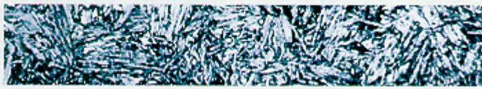
Too high hardening temperature gives coarse structure, high austenite content (30%), few carbides.
